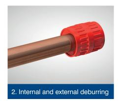
The tubes should then be carefully deburred inside and out to remove all sharp edges and debris.
