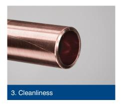
Once the tube has been prepared, check for any deep scratches and scores in the tube. If either are visible cut the tube back and start the process again.
