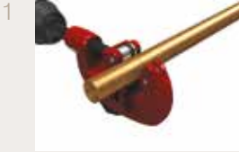
Cut tube to length required
