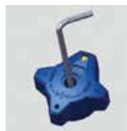
C) Take off the green cap on the handwheel. Using a 4mm Allen key turn the memory device clockwise until it stops, the maximum opening position is set to 2.5 turns.
