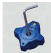
C) Take off the green cap on the handwheel. Using a 4mm Allen key turn the memory device clockwise until it stops, the maximum opening position is set to 2.5 turns.
