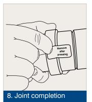
· Remove the actuator from the press ring, remove the press ring from the tube and remove the label to indicate the joint is pressed and complete.
