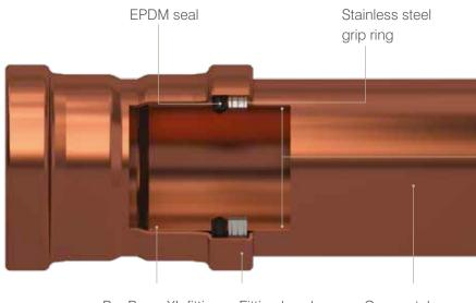
The action of the pressing ring closes the joint and forces the grip ring teeth into the tube making a high strength connection.
