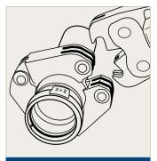
6. Engage the actuator and check insertion depth
