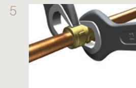
5 Tighten joint to the correct number of turns as per recommendations stated in the technical catalogue
