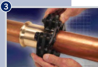
**3** Ensure that the groove in the collar corresponds to the bead on the fitting and that the support plate on the collar fits over the tube side of the joint.
