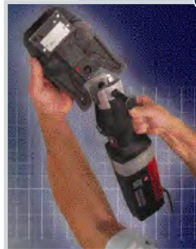
**6** Depress the button on the press tool and begin the pressing operation.
