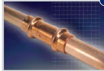
**2** Using the correct sized jaws in the press tool, place them over the bead at the mouth of the fitting. Maintain a 90° angle between tube and jaws to ensure a sound joint is made.
