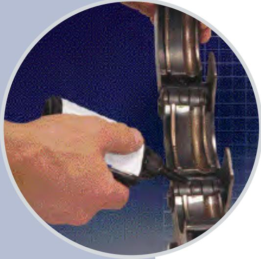
We recommend the use of press collars rather than two-piece jaws when jointing larger size fittings. The collars provide an equally distributed pull around the circumference of the fitting. For 108mm red brass fittings a secondary press is undertaken to ensure a sound joint.
