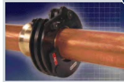
**5** Take the appropriate adaptor and attach to the press tool, then close the breach bolt. To attach the collar, depress the jaw levers and attach the claws as far as you can into the grooves of the collar. Unless the adaptor is correctly connected to the press collar pressing will not be possible.
