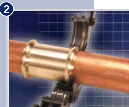
**2** Select the appropriate collar and open by depressing the spring loaded pin. Pull apart and position over the fitting.
